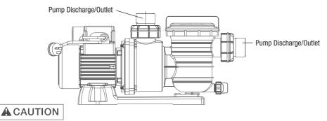
The fittings on these pool pumps are constructed of ABS. Some PVC jointing compounds are incompatible with ABS possibly causing failure to the product. Check compound suitability prior to use.
