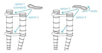
• **Extended Float Bar** (optional) – fits to either the top or bottom bridge to adjust the VTX-7's turning circle.
