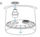
**NOTE:** A Vacuum Plate Clamp can stop your vacuum plate moving. **TIP:** The Anti-Vortex Washer stops the slurping sound.
